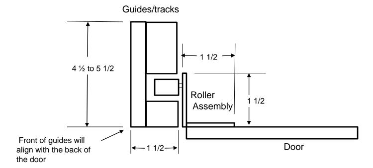
NOTE: Custom roller assembly designs are available. Also, wood extensions for the roller assembly can be made so that he guides can be moved out further too the left and the right to better conceal them from the door opening
