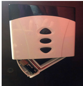
Wireless wall switch (remote) Showing battery access
